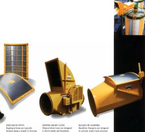
located along a length of ducting, however may also be applied to dust collection or storage equipment. They are designed to burst open at a predetermined pressure increase, reducing the damage caused by an explosion. When the pressure inside the duct work or vessel increases, the aluminum diaphraem relieves on three (3) sides. The fourth side of the diaphragm is secured with bolts to prevent it from becoming air borne.
